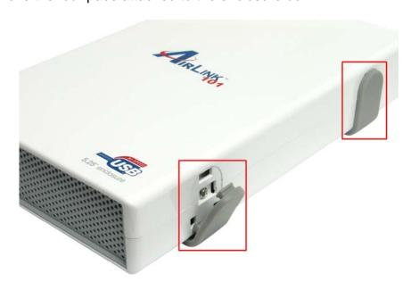
Step 2 Use the provided screwdriver to remove the screws on each side of the box.
